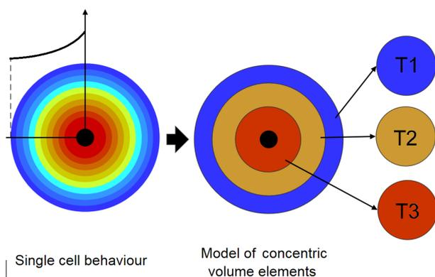
**Figure 1: Cylindrical cell with continuous radial temperature distribution approximated as series of concentric elements electrically connected in parallel.**
