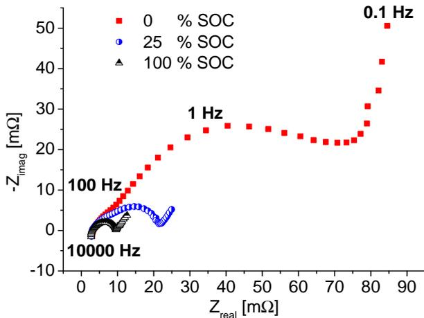
Fig. 12. NMC cell impedance variation with SOC
