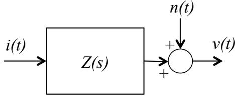
Fig. 3. Impedance represented as a transfer function
