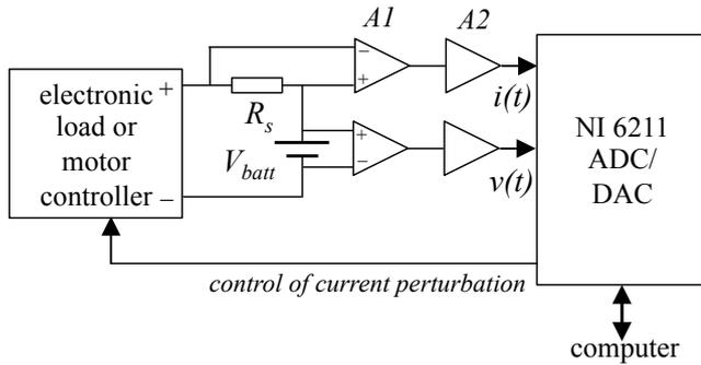
Fig. 4. Impedance measurement system for a single cell
