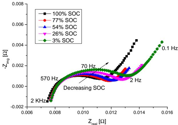
Fig. 2. Variation in LFP cell impedance with SOC (x-axis shows real part of impedance, y-axis shows negative reactive part)
