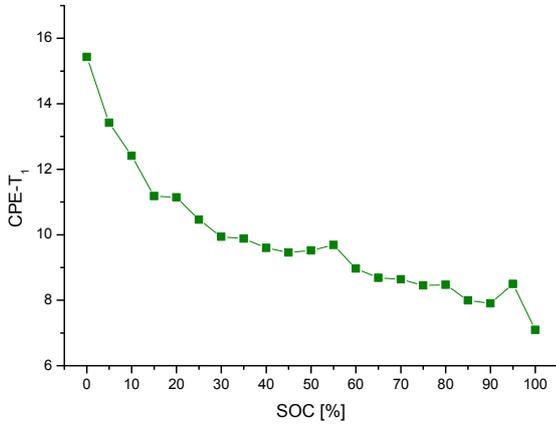
Fig. 11. Constant phase element CPE1 variation of admittance  $T_1$  with SOC
