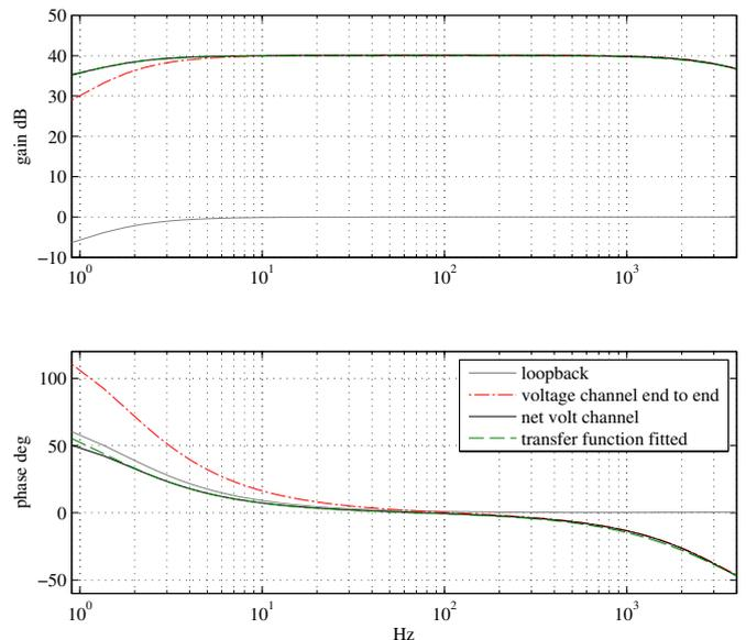
Fig. 5. Voltage channel measured response using network analyser
