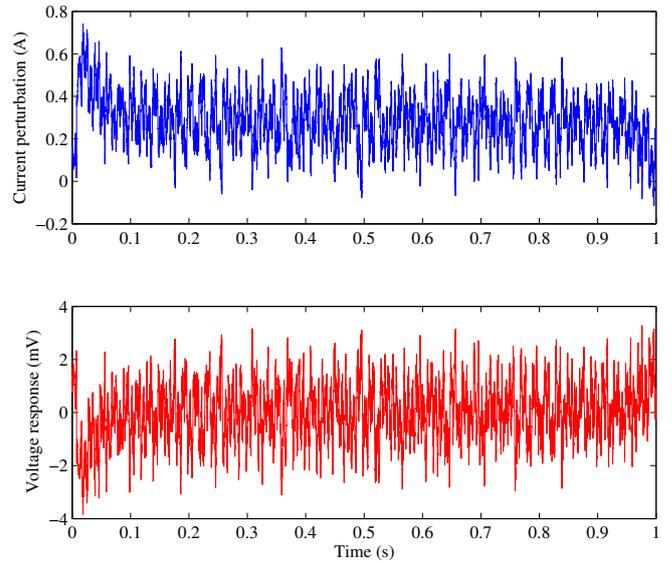
Fig. 6. Measured current and voltage, single cell with multi-sine excitation
