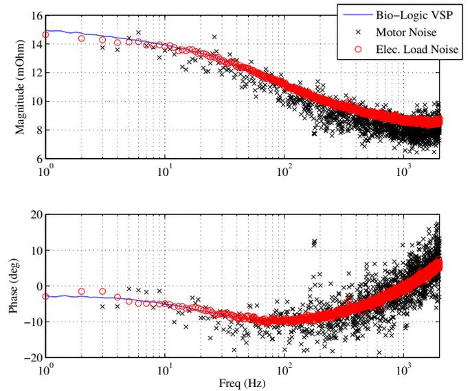
Fig. 8. Measured impedance comparison using broadband noise excitation
