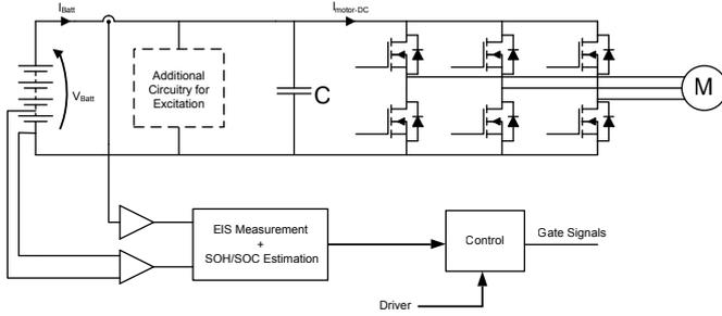
Fig. 1. Battery impedance measurement within vehicle drivetrain
