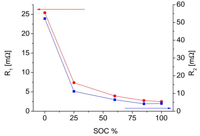
Fig. 13. SEI resistance  $R_1$  and charge transfer resistance  $R_2$  variation with SOC for NMC cell
