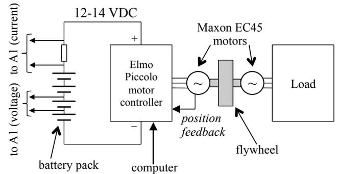
Fig. 9. Motor controller battery test system with 4 cells. Only one battery voltage measurement plus the current shunt is shown.
